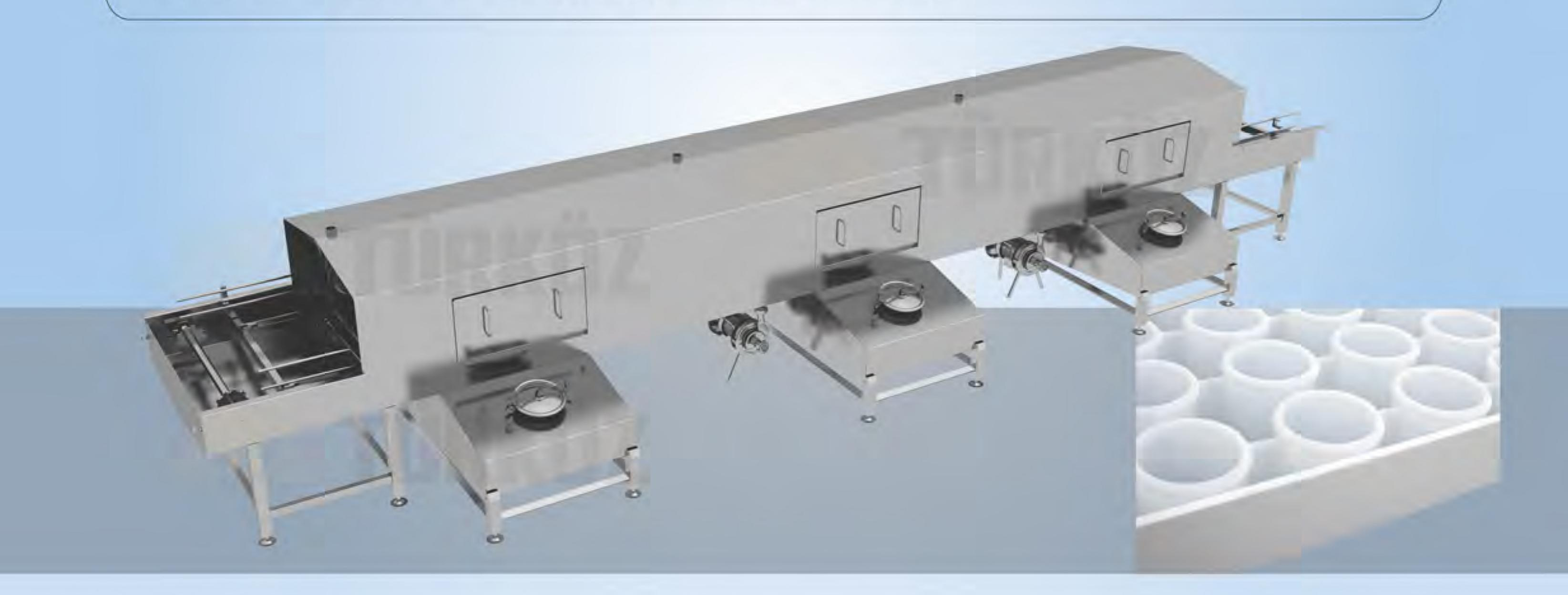
Mould draining conveyor operates in coordnation with main system. It carries cheese mould automaticaly. This machine has no standart length or width. Dimensions are determined accordingly capacity of facility.
