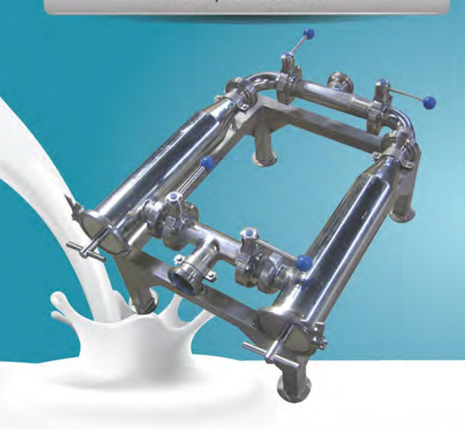
It is the equipment to initial device to receive milk to facility at first. Inside and outside of it is made of stainless steel. Filter's micron value of device can be chosen. It is easy to remove and clean it. What Türköz company recommends is to have double fitler system. Advantage of double filters is if one of them is jammed the other one will go on to work.
