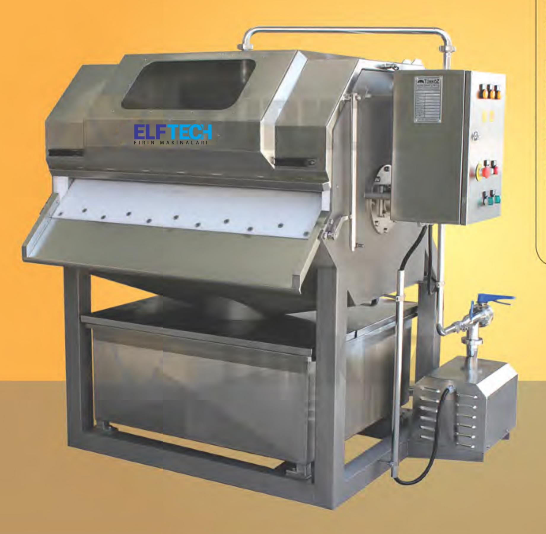
Modern drums systems are generally used for high capacity process tanks. Cheese to be filtered is transfered forward over top side of drums. Comparing to conventaional drums perforations can be smaller. Drum speed can be adjusted. Whey is collected in a tank which is placed beneath drum. Transfer to any place desired can be done with high-pressure pumps. As the system has wheels and mobile it can be used with various tanks in facility. Drum is designed compatible with CIP system.
