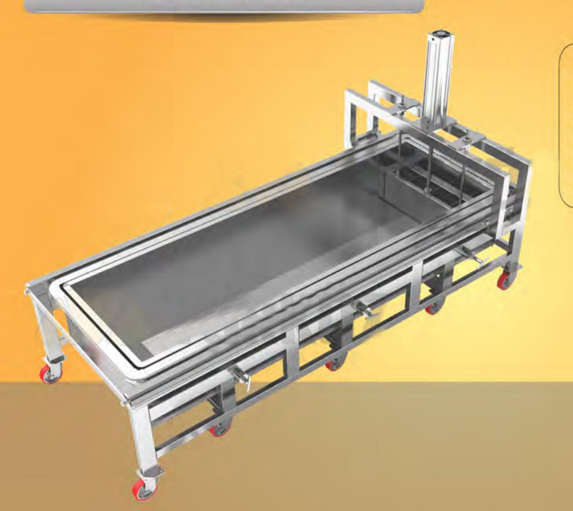
This equipment is used to portion special types of cheese. This equipment Works with pressing system. After pressing cheese are transfered to cheese cutting. Cheese is cut in different portions depending type of knives. As it has wheels, system can be moved anywhere.
