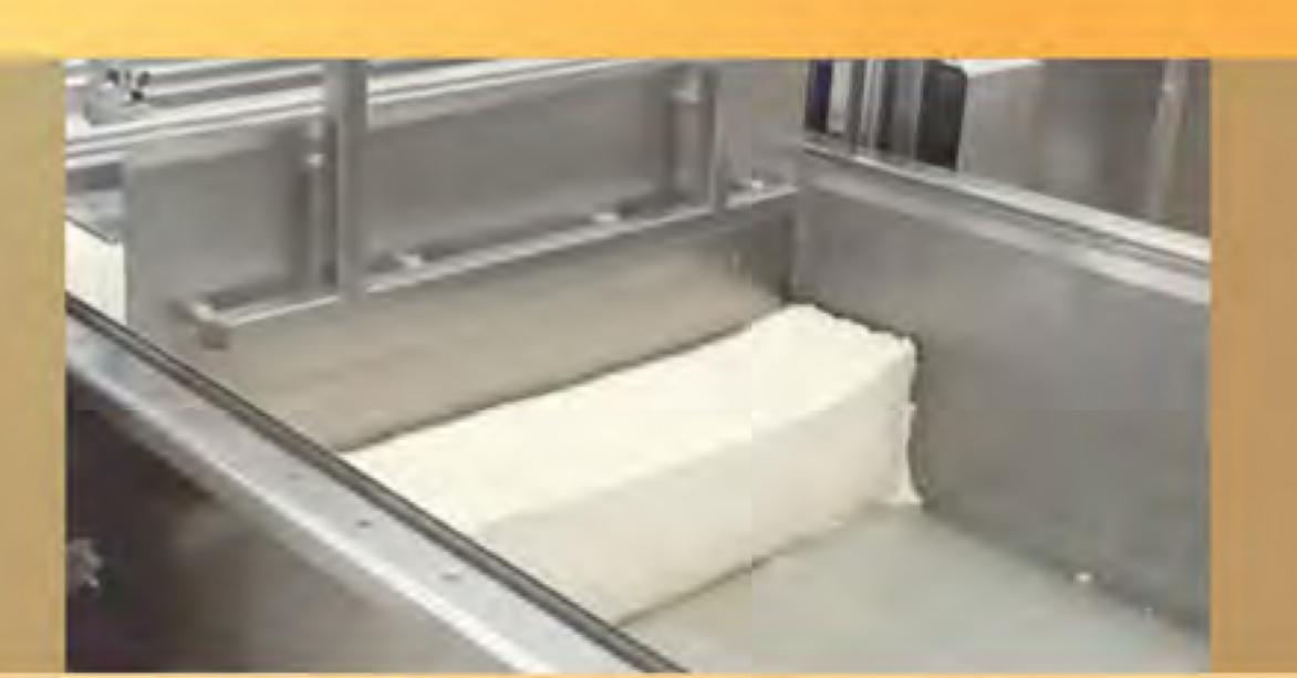
Curd cheese cutting and transferring machine cuts curd cheese which has stable pH value and transfers it to cooking machine through augers without human contact. Machine is designed entirely closed system. And it can easily be cleaned with CIP system.
