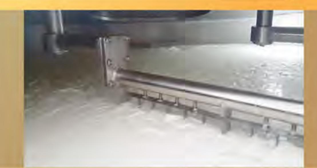
If cheddaring system is used there will be no need for drums for filtering. Both cheese coming out from process and its whey are mixed in cheddaring system to keep it fresh and then whey is filtered. So pH value and amount of dry matter within products is standardized. With standart and stable values process more balanced and productive. This vat also provides transfering curd cheese without human contact. Cheddaring system's capacity may vary depending capacities of process tanks.
