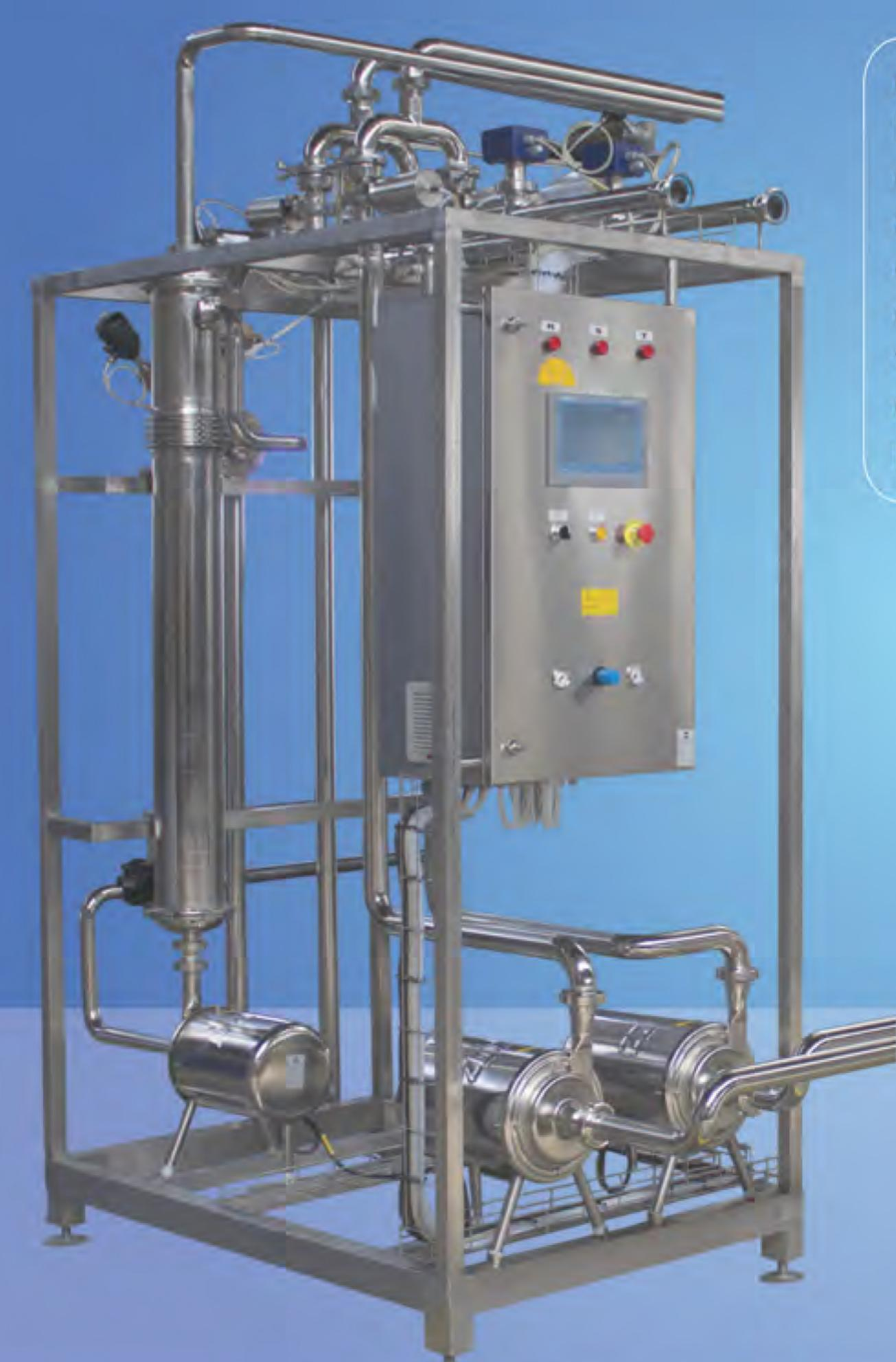
Control unit, contains electric panel, pumps, valves and heating exchangers of CIP system. Control units provides connection between CIP tanks and lines to be washed and also reports about process. System can be controlled over touch screen. All phases of cleaning can be observed on screen. This unit can control temperature, conductivity, level, flow and timing. It also can adjust dosing so that chemical loss is minimum. Thanks to reportability all posibble mistakes are eliminated.
